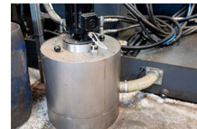
This is our high-end external machine connection which is necessary for some applications like when your working with aluminum chips.
