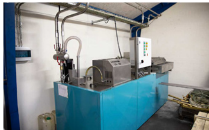
The central filtration system for filtering the lubricant.
